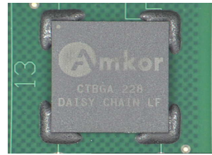
Figure 1: An example of an edge-bonded CSP.
