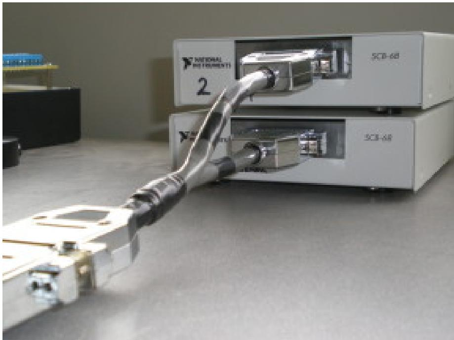
Figure 2.7: NI Connector boxes with spliced cable connected
